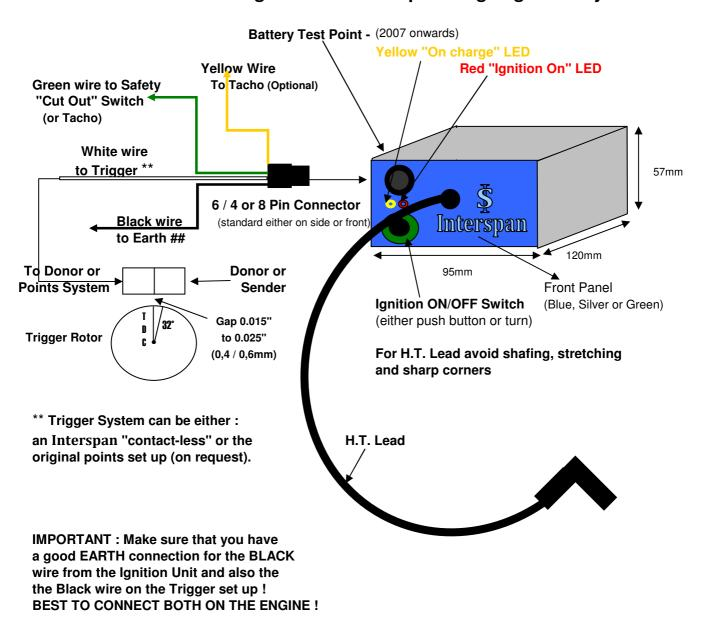
Please Remember: Switch OFF the Ignition Unit BEFORE connecting the 12v Charging supply!
